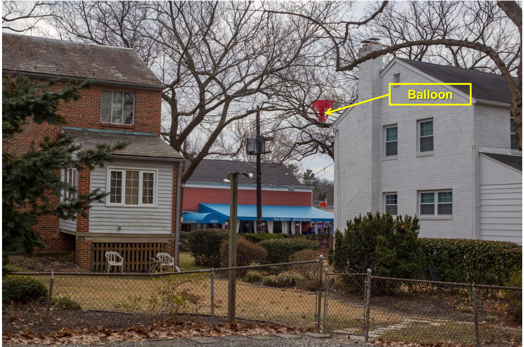
View from Camera Loc. 04. The 3D model-massing accurately represents the visual impact of the proposed development from this alley perspective between Yuma and Alton. Belly of balloon is located at 51ft (height of terrace). Total building height is 89 feet.
