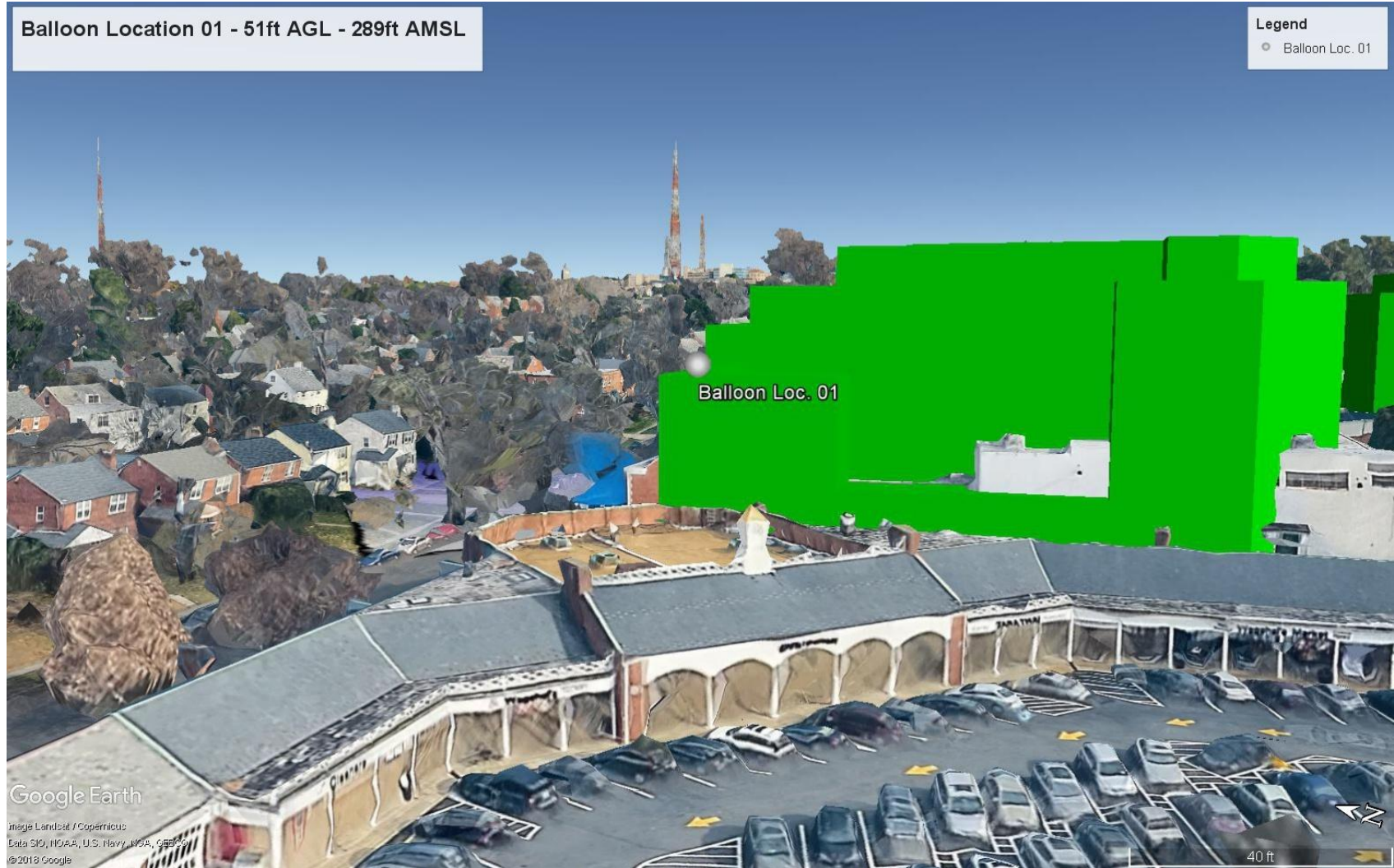
Illustration shows the DDIS tethered aerostat balloon at the North end of alley. Laser range finders were used to verify the balloons height at 51ft height and its horizontal location of the proposed building terrace.
